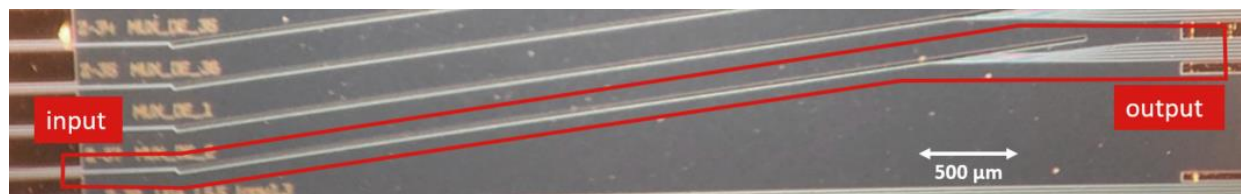
Fig. 3. Microscope photo of the angled MMI (de)multiplexer with five channels.
