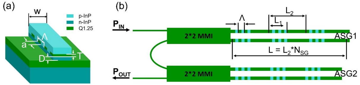
Fig. 1. (a): Schematic diagram of uniform DBRs in SMART Photonics platform. The layer stack has been simplified, without showing doping differences in p-InP and n-InP layers. (b): Schematic diagram of the top view of tunable filter.
