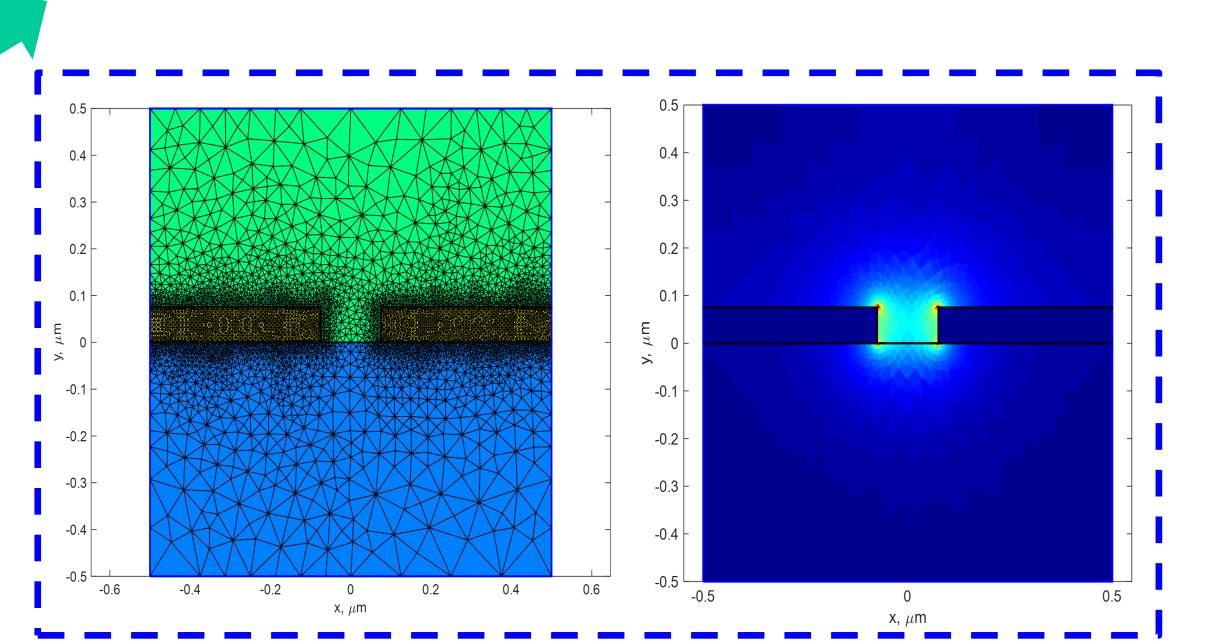
The refractive index change is used as input of the optical waveguide simulator, which estimates the mode features of the waveguides. E/O effect is enhanced by the stronglylocalized plasmonic mode (left, optical mesh; right, fundamental plasmonic mode)
