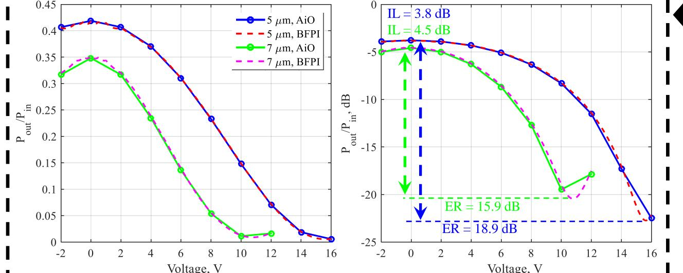
The results obtained with all-in-one 3D-FDTD simulations (AiO) are compared to those achieved with the bimodal Fabry-Pérot interferometer model (BFPI) for two devices having 5 µm (blue/red curves) and 7 µm modulator length (green/magenta curves).
