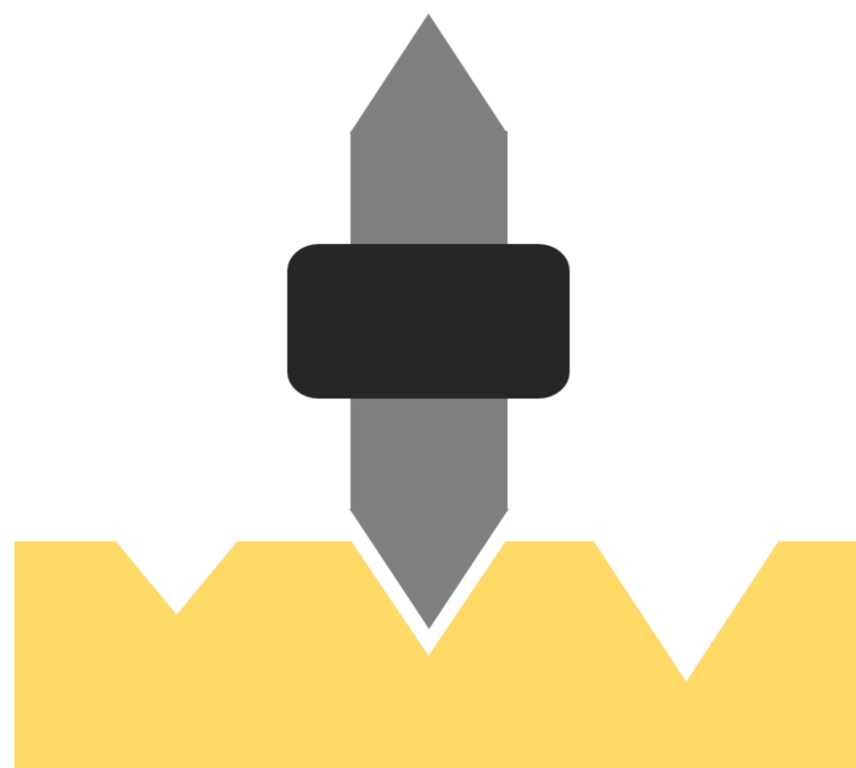
Figure 1. Illustration of V-shaped wheel and different depth V-groove cuts on lithium niobate sample.
