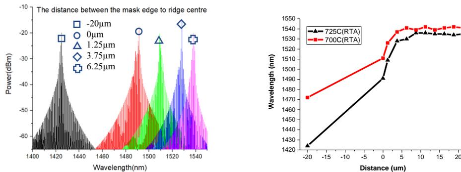
Figure 7. The lasing spectra of the FP laser annealed at 725°C with different distance between the ridge centre to the edge of the QWI mask (left). Figure 8. The lasing peak wavelength vs the distance between the ridge centre to the edge of the QWI area mask (all the FP lasers are tested under 40mA and the same other condition). Here, "-20" and "0" represent the ridge is in the centre of the mask and half covered by the mask (right).
