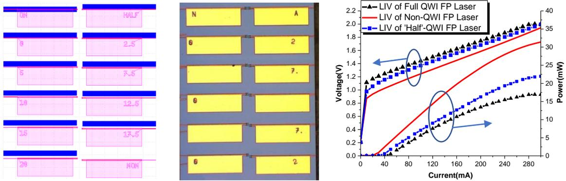
Figure 4. 12 lasers with different distances (the numbers on the chip design represent the distance from edge of the mask to the edge of the ridge) on the QWI boundary (left) and Figure 5. Microscopic picture of the fabricated FP lasers array (middle). Figure 6. Characteristics of current-voltage and output power-current at 20°C of non-QWI FP laser, 'Half'-QWI FP laser and Full-QWI FP laser (right).
