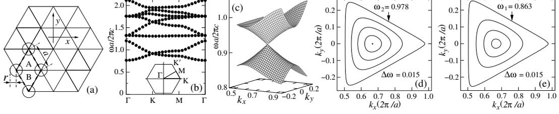
Figure 1. Triangular photonic structure (a) and the corresponding EM frequency band diagram (b). A 3D view of the Dirac cone at K ( $4\pi/3a, 0$ ), formed by the first two bands, is shown in (c). Iso-frequency contours of the upper and lower cone at the same K point are depicted in (d) and (e), where the frequency level ( $\omega_1$  and  $\omega_2$ ) as well as the contour interval ( $\Delta\omega$ ) values are normalized to  $\omega a/2\pi c$ .
