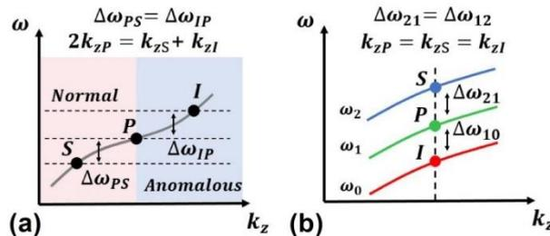
Fig. 1. Description of the degenerate four wave mixing process operated in a single-mode waveguide with anomalous dispersion (a) and operating within an inter-modal scheme regardless the absolute dispersion provided that all dispersion curves are obtained by translating the same curve with a constant frequency step (e.g.  $\Delta\omega_{21}=\Delta\omega_{10}$  here).
