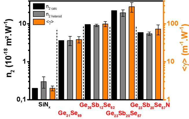
Figure 1: Experimental nonlinear coefficient  $\gamma$  of some chalcogenide thin films and SiN<sub>x</sub> measured in waveguides at 1550 nm. The  $n_{2\text{ heterod}}$  Kerr index is deduced from nonlinear coefficient and compared to  $n_{2\text{ calc}}$  the Kerr index calculated using the Sheik-Bahae model.
