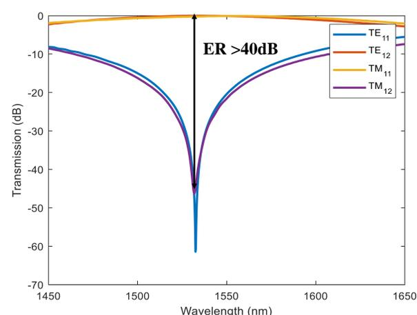
Figure 2. Simulation of ideal polarization splitter.  $w_1 = 1.58 \mu\text{m}$ ,  $w_2 = 2.5 \mu\text{m}$ ,  $L_1 = 236.5 \mu\text{m}$ ,  $L_2 = 793.6 \mu\text{m}$ ,  $w_0 = 13.5 \mu\text{m}$ , and  $L = 216 \mu\text{m}$  is used for simulation.
