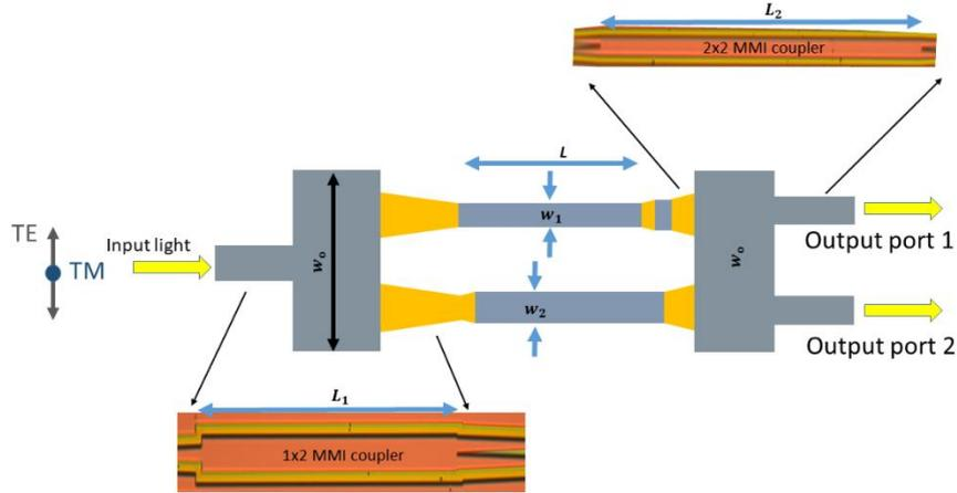
Figure 1. Schematic and microscopic pictures of polarization splitter based on Mach-Zehnder interferometer design.
