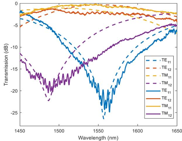
Figure 3. Analytical model results compared with measurement results. The dotted lines present the simulation results and straight lines present the measurement results.
