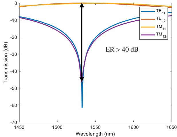
Figure 2. Simulation of ideal polarization splitter.  $w_1 = 1.58 \mu\text{m}$ ,  $w_2 = 2.5 \mu\text{m}$ ,  $L_1 = 236.5 \mu\text{m}$ ,  $L_2 = 793.6 \mu\text{m}$ ,  $w_0 = 13.5 \mu\text{m}$ , and  $L = 216 \mu\text{m}$  is used for simulation.
