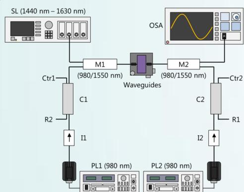
PL: Pump Laser, I: Isolator, R: Residual Pump, C: Coupler, Ctr: Pump Control, M: Multiplexer, SL: Signal Laser, OSA: Optical Spectrum Analyzer.
