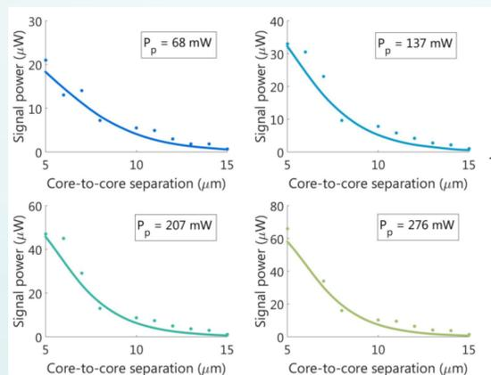
Output signal power dependence on core-to-core separation, for different unidirectional pump powers
