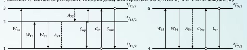
being  $W_{ij}$  the stimulated transition rates and  $A_{ij}$  the relaxation rates between  $i$ th and  $j$ th levels,  $C_{tr}$  and  $C_{inv}$  the direct and inverse energy transfer rates and  $C_{up}$  the homogeneous upconversion coefficient. Some of the parameters needed in the theoretical model must be obtained experimentally. In order to do that, we first characterize an isolated waveguide written in the same bulk glass.
