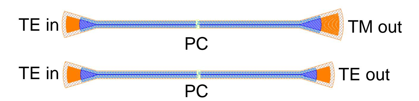
We introduce a new 4-port measurement method. The structures used for the measurements are shown below. The characterization is done by doing four measurements, which are the transmitted powers  $P_{13}$ ,  $P_{14}$ ,  $P_{23}$ ,  $P_{24}$ :
