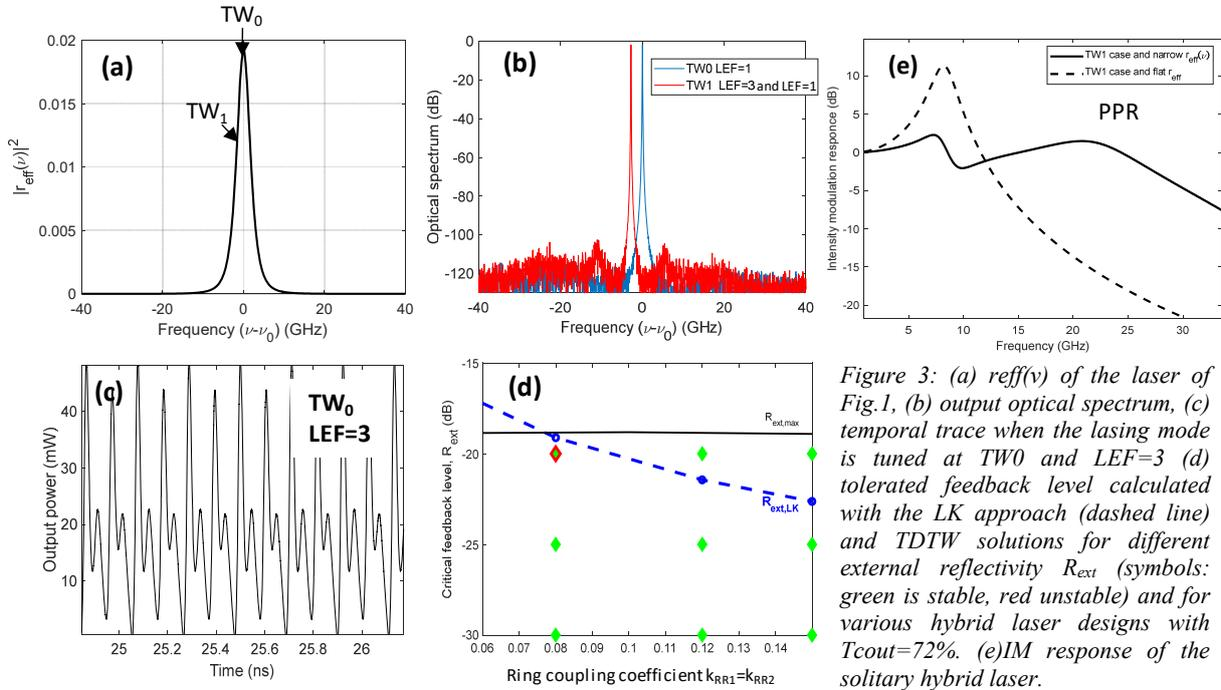
Figure 3: (a)  $r_{eff}(\nu)$  of the laser of Fig.1, (b) output optical spectrum, (c) temporal trace when the lasing mode is tuned at  $TW_0$  and  $LEF=3$  (d) tolerated feedback level calculated with the LK approach (dashed line) and TDTW solutions for different external reflectivity  $R_{ext}$  (symbols: green is stable, red unstable) and for various hybrid laser designs with  $T_{coul}=72\%$ . (e) IM response of the solitary hybrid laser.
