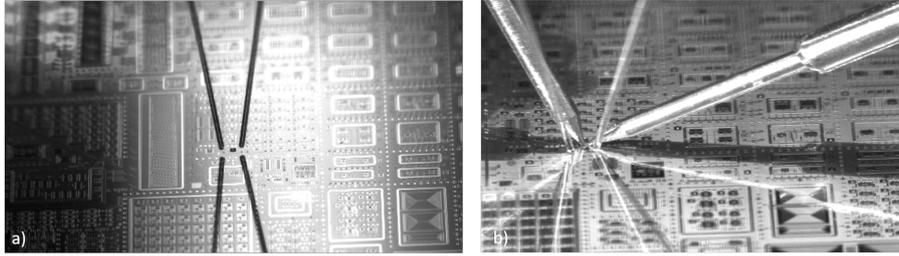
Figure 3. a) Camera picture of a cavity with deposited LC between two cleaved fibres.(b) Measurement setup, with electrical probes for the actuation and aligned optical fibers to vertical grating couplers to measure the MZI transmission spectrum.
