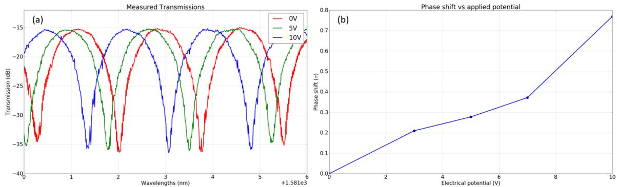
Figure 4. (a) Measured MZI responses for applied potentials of 0 V, 5 V and 10 V. (b) Phase shift for different applied voltages.
