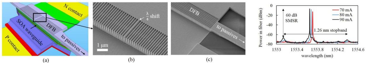
Fig. 5. DFB-laser. From left to right: schematic, DFB-grating, output connection, spectrum.
