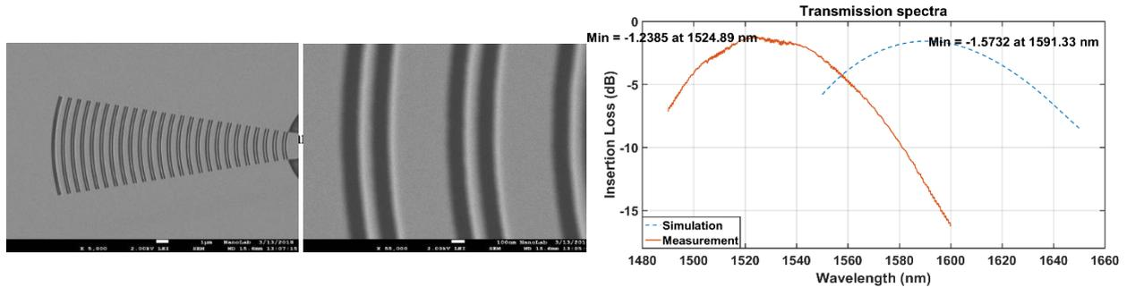
Fig. 4. Grating coupler using apodization, sub-wavelength structuring and a metal back reflector. Left: transmission spectra.
