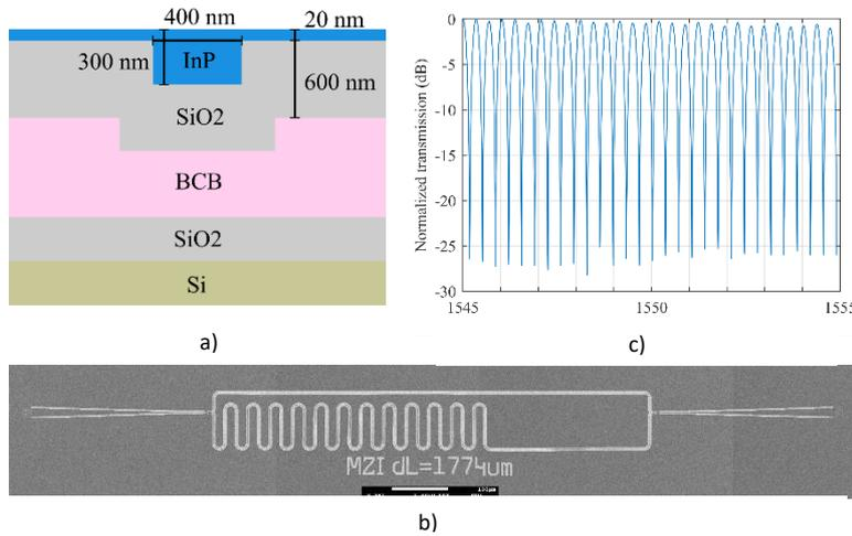
Fig. 2. Results from wafer scanner lithography. a) Cross-section of IMOS waveguide, b) MZI-structure for loss measurement, c) spectral response of the MZI.
