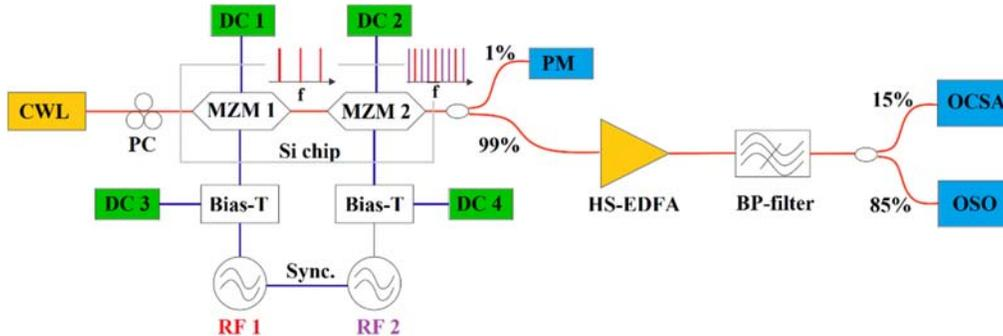
Figure 3. Experimental setup of on-chip OFC generation. CWL: continuous wave laser, PC: polarization controller, RF: radio frequency, DC: direct current, PM: power meter, HS-EDFA: highly sensitive Erbium doped fiber amplifier, BP-filter: bandpass filter, OCSA: optical complex spectral analyzer, OSO: optical sampling oscilloscope.
