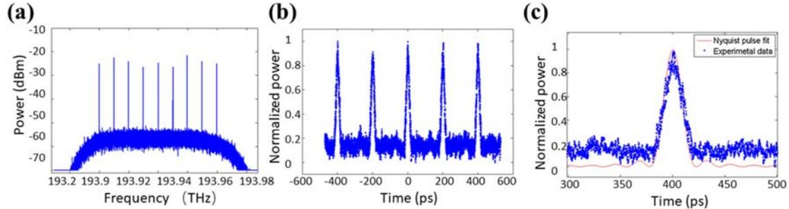
Figure 5. Measured spectrum (a) and time-domain waveform (b) of a comb with 9 lines and a spectral separation of 5 GHz; (c) curve fit of measured time-domain waveform using sinc-shaped Nyquist pulse.
