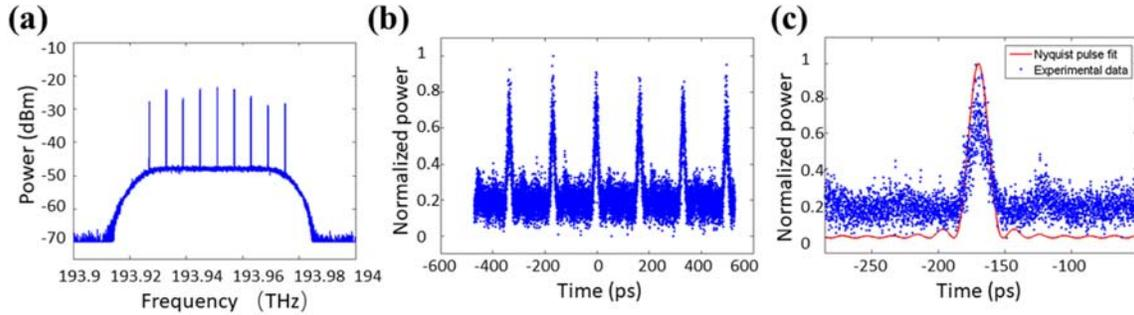
Figure 4. Measured spectrum (a) and time-domain waveform (b) of a comb with 9 lines and a spectral separation of 6 GHz; (c) curve fit of measured time-domain waveform using sinc-shaped Nyquist pulse.
