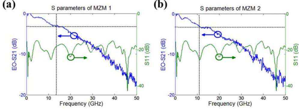
Figure 2. Measured  $S_{11}$  and  $S_{21}$  parameters of (a) MZM1 and (b) MZM 2.
