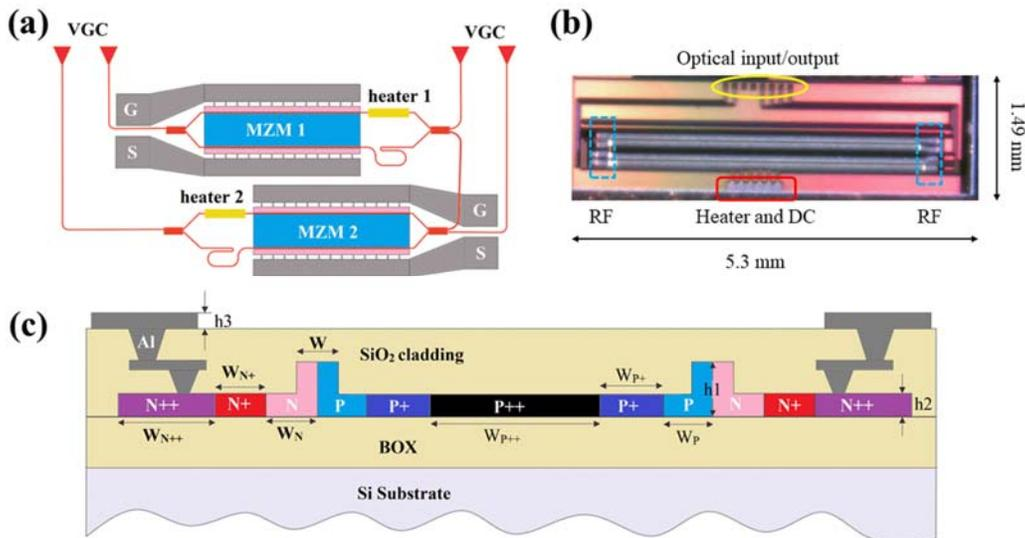
Figure 1. (a) Device schematic, (b) photo of fabricated device, and (c) cross section of push-pull MZM. The dimensions are:  $h_1=500$  nm,  $h_2=90$  nm,  $h_3=2$   $\mu$ m,  $W=500$  nm,  $W_{N^{++}}=5.2$   $\mu$ m,  $W_{N^+}=0.81$   $\mu$ m,  $W_N=0.39$   $\mu$ m,  $W_{P^{++}}=28$   $\mu$ m,  $W_{P^+}=0.83$   $\mu$ m,  $W_P=0.37$   $\mu$ m.
