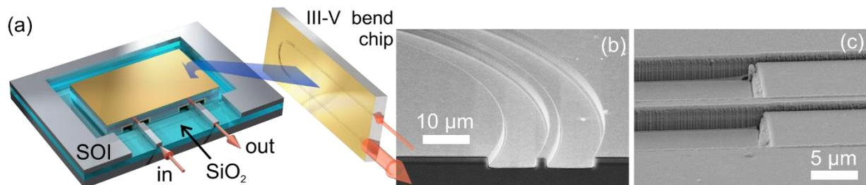
Figure 1. (a) Integration of III-V semiconductor chip with U-bend geometry on silicon-on-insulator (SOI) chip. The I/O ports are on the same side of the chip thus alleviating the requirement for precise dimension control of the chip. (b) Scanning electron microscope (SEM) image of the bend. (c) SEM image of the step between the bent and straight RWG.
