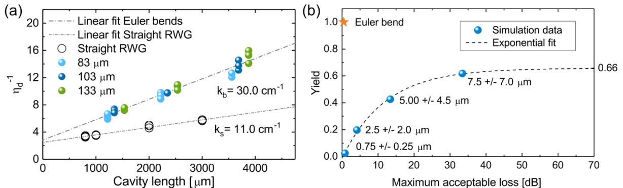
Figure 2. (a) Inverse of the differential quantum efficiency plotted as a function of cavity length for U-bend and straight waveguide devices. (b) The yield of the traditional straight waveguides tilted 7° as a function of the simulated coupling loss.
