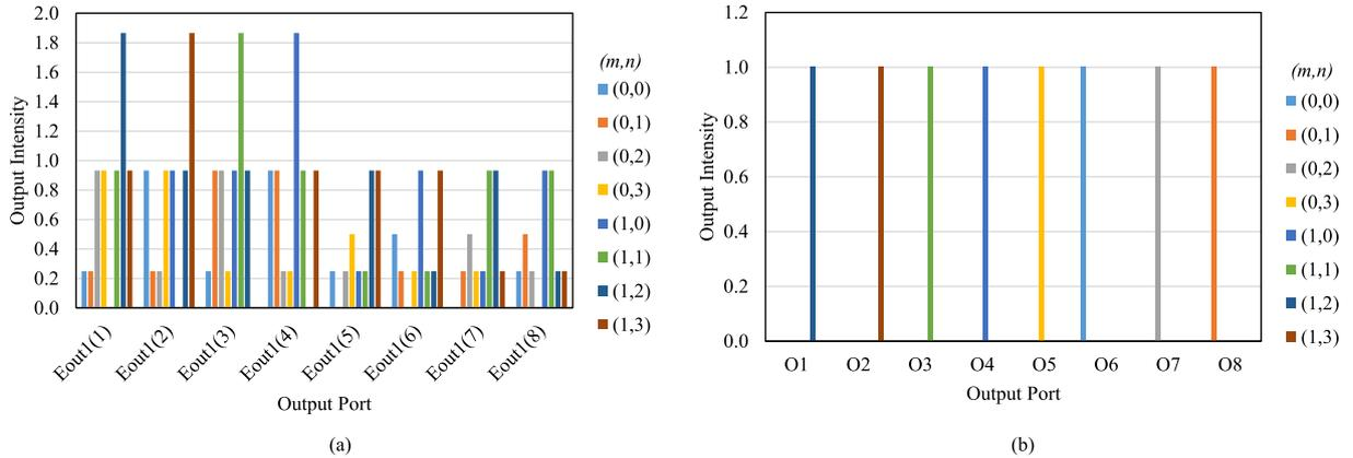
Figure 4. Output intensities (a) before thresholder and (b) after post processing logical circuit.
