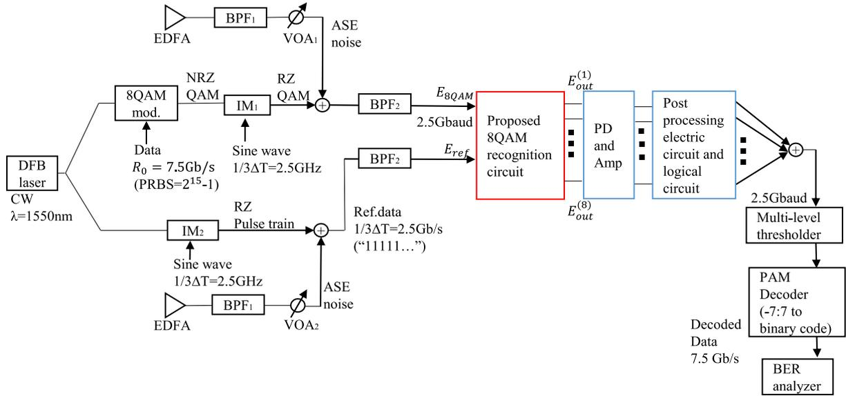
Figure 5. A simulation set-up for noise tolerance.
