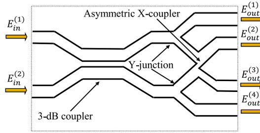
Figure 2. QPSK code recognition circuit.
