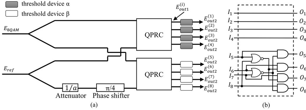
Figure 3. (a) Proposed 8QAM recognition circuit by the maximum output, (b) Post-processing logic circuit.
