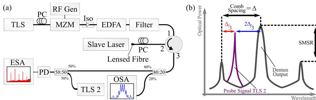
Figure 1. (a) The experimental setup used to perform the comb experiments. TLS: Tunable laser source, MZM: Mach zehnder modulator, PC: Polarisation controller, EDFA: Erbium doped fibre amplifier, OSA: Optical spectrum analyser, PD: Photodiode, ESA: Electrical spectrum analyser. (b) Illustration showing where the probe wavelength from the second TLS was located relative to the demultiplexed comb.
