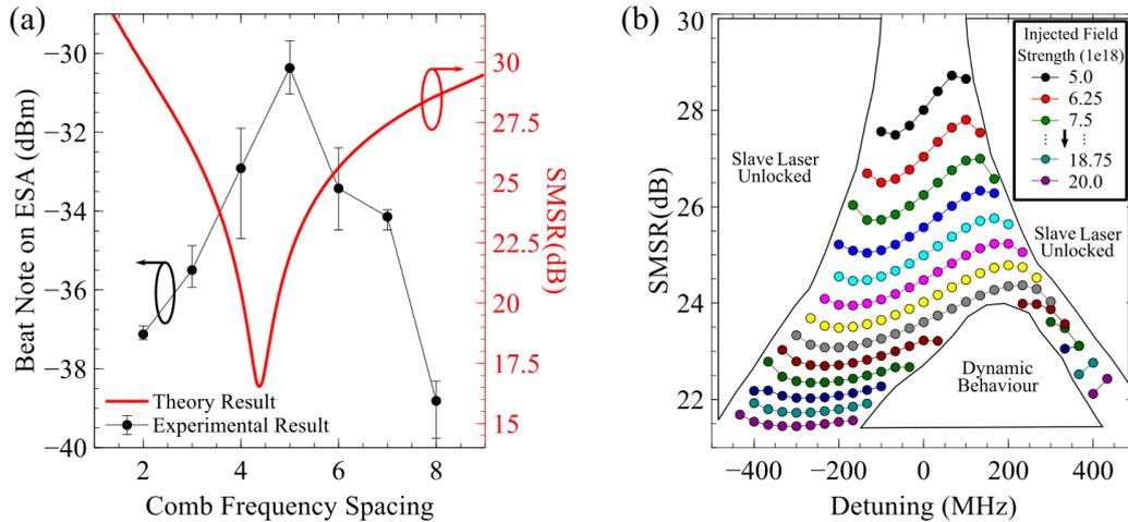
Figure 2. (a) Experimental results (left axis) showing the beat note of the unlocked comb line with the probe TLS versus comb spacing, with an inject power of  $-8$  dBm. Simulated SMSR (right axis) results for an injected field strength of  $2.1 \times 10^{18}$ , at 1.33 times threshold. (b) Simulated SMSR versus detuning. From top to bottom, optical power increases in steps of  $1.25 \times 10^{18}$  for a  $10$  GHz spacing.
