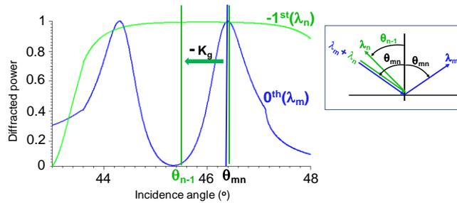
Figure 3 Angular spectra at  $\lambda_m = 1510$  nm and  $\lambda_n = 1525$  nm with  $\Lambda = 732$  nm,  $w_g = 275.264$  nm,  $h = 279.3$  nm. The  $\lambda_m$  channel is reflected forward. The  $\lambda_n$  channel is diffracted back by the  $-1^{\text{st}}$  order grating constant  $-K_g$  under the angle  $\theta_{n-1}$ .
