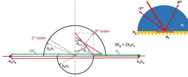
Figure 1 Ewald circles in the spatial frequency domain illustrating the conditions on the incidence angle in the medium of high index  $n_i$  for the total reflection of all diffraction orders while the +1<sup>st</sup> and -2<sup>nd</sup> grating orders excite the forward and backward propagating waveguide mode. The inset is an example of a monolithic device in the direct space.
