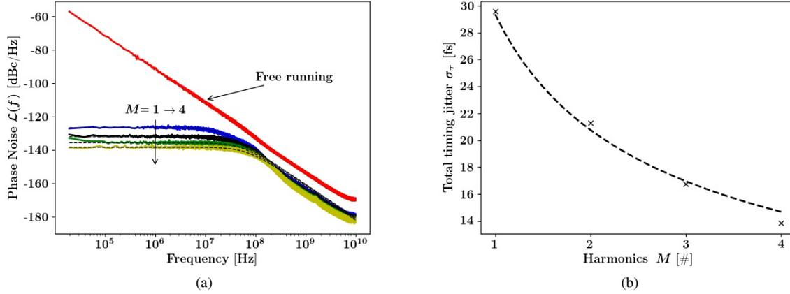
Figure 3. (a) Phase noise of free running and hybridly MLL. (b) Total timing jitter computed from fitted curves in (a).
