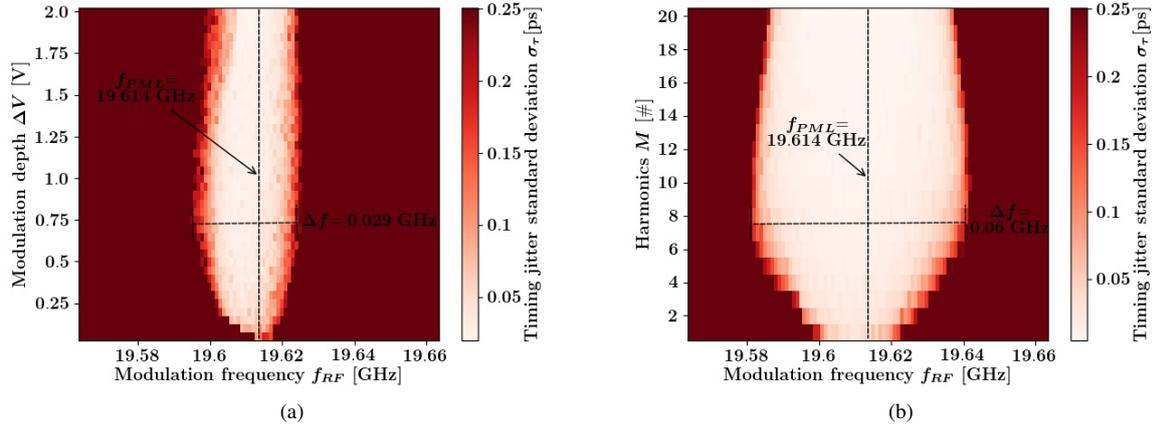
Figure 2. Locking range map based on timing jitter standard deviation in a 750 ns interval, for (a) increasing modulation depth and (b) increasing number of harmonics. Values above the free running timing jitter standard deviation 0.25 ps have been rounded to this value.
