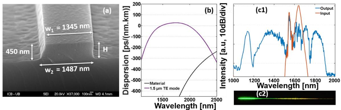
Figure 2. (a) Scanning Electron Microscope image of the cleaved strip waveguide (b) Dispersion properties for the fundamental TE<sub>0,0</sub> mode. (c1) Optical supercontinuum obtained at the output of the waveguide (solid blue line) compared to the input pulse spectrum (red solid line). (c2) Image of the emitted visible light from the waveguide (total length ~ 6.5 mm).
