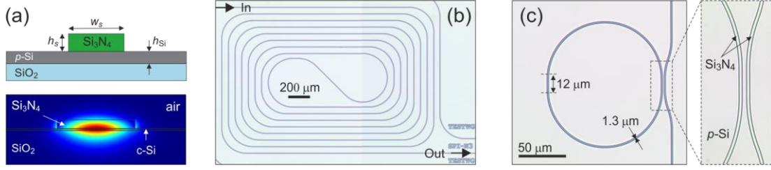
Figure 1. (a) The cross-sectional view of the waveguide and the distribution of the simulated electric field intensity of a transverse electric (TE)-polarized mode. Optical micrographs of a typical (b) spiral waveguide and (c) a ring resonator.
