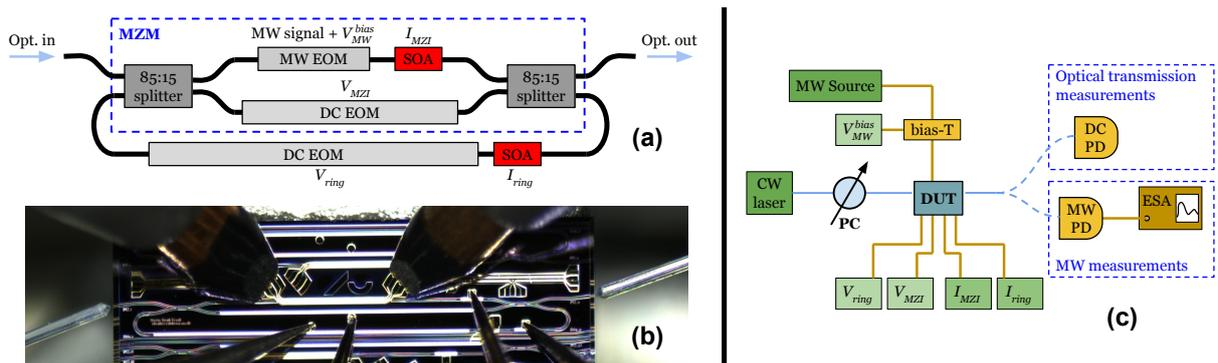
Figure 1. (a) Schematic of the ring resonator MW modulator. (b) Microscope image of the fabricated modulator with DC/MW probes and edge coupled fibers. (c) Measurement setup to obtain either the optical transmission or the MW response.
