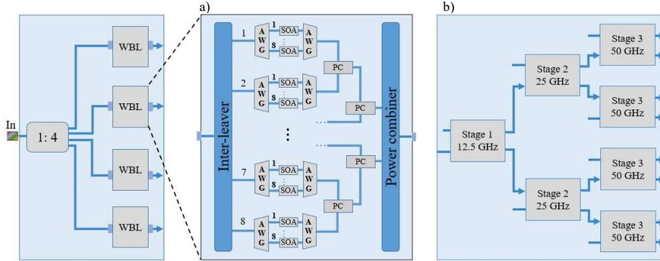
Figure 1: Architecture of the  $1 \times 4$  fast WSS and detail of (a) one of the four  $64\text{-}\lambda$  WBL prototypes and (b) the 1:8 interleaver
