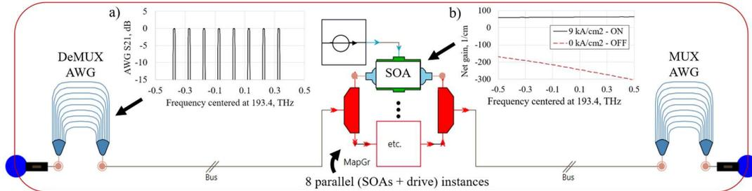
Figure 2: MUX-DEMUX unit setup including a current-driven SOA per AWG channel with detail of (a) the AWG transfer function and (b) the gain of the SOAs in the 'on' and 'off' state.
