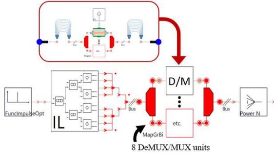
Figure 3: 64- $\lambda$  WBL simulation setup including a 1:8 interleaver (IL) and 8 parallel DeMUX/MUX (D/M) units
