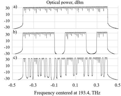
Figure 4: Steady-state transfer characteristic of the WBL (a) at max gain, (b) with 4th and 7th SOA-channels switched off, and (c) with arbitrary slicing drive.
