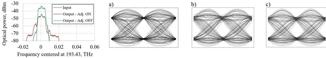
Figure 5: Signal spectra of the WBL 10 Gbd input and output signals with eye diagram detail of a) the input signal, b) the output signal with adjacent slices on, and c) the output signal with adjacent slices off.
