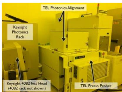
Figure 3. Newly installed electrical optical test equipment in the SUNY Poly cleanroom. The tools, part of the Inline Test Development project, will reduce the time to detect a misprocessed wafer from 4 months to a few days. Credit: AIM Photonics
