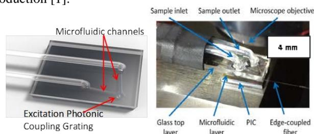
Figure 2. Schematic (left) and fabricated device (right) for microfluidic-enabled PIC for SERS. Credit: Carl Meinhart, University of Rochester.
