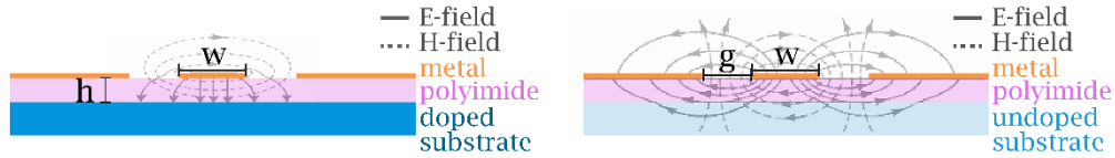
Figure 1: Microstrip (left) and coplanar waveguide (right) transmission line behaviour, with the important parameters for their design.
