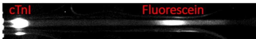
Figure 3. Fluorescence microscopy image of an experiment where cardiac troponin I (cTnI) and fluorescein are separated and concentrated. Results obtained at BIOS Lab-on-a-chip group at the University of Twente.
