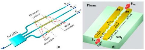
Fig. 2. (a) Silicon-based biosensing platform with (b) a zoom of the plasmonic cavity as sensing element [10]
