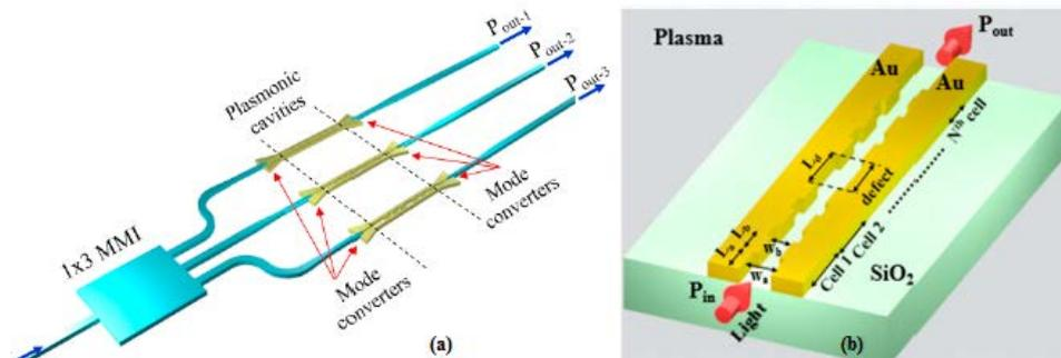
Fig. 2. (a) Silicon-based biosensing platform with (b) a zoom of the plasmonic cavity as sensing element [10]
