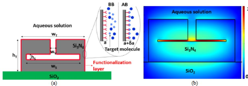
Fig. 1. (a) Cross-section of the waveguide of the slotted MRR configuration and (b) fundamental quasi-TM mode distribution.
