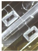
Fig. 2 Microscopic topview image of propagation through a fabricated optofluidic device.
