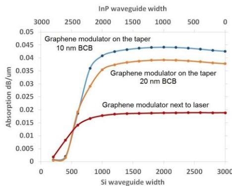
**Fig. 2. The TE mode absorption as function of the InP taper width and Si waveguide width for two designs of graphene modulator next to laser and graphene modulator on the tapered Si integrated with laser.**
