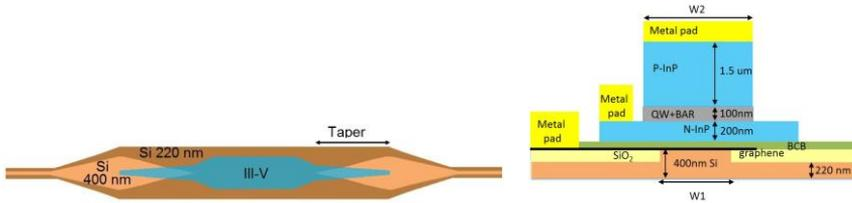
**Fig. 1. Left: III-V on Si laser design, top view, Right: Schematic of the graphene device integrated with an InP/Si laser. The structure is on the taper section in the left image, therefore the width of Si waveguide and P-InP is varied.**
