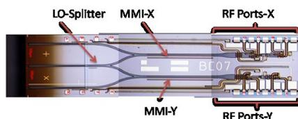
**Fig. 2. Dual polarization coherent receiver chip on InP comprising spot-size converters, power splitters and optical mixers and 8 photodiodes.**
