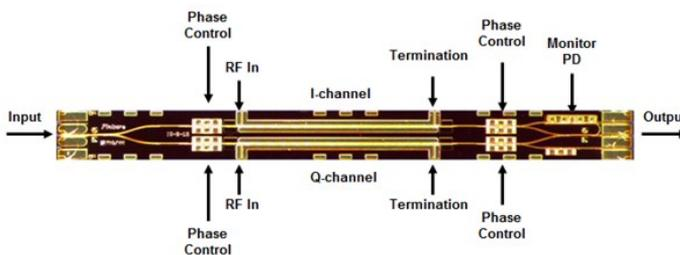
**Fig. 3. I-Q modulator PIC on InP, comprising two nested MZMs, monitor PDs, phase control sections and electrical termination.**
