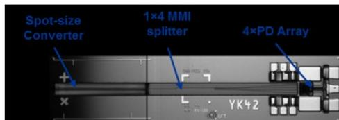
**Fig. 1. Four waveguide integrated photodiodes coupled to a 1x4 MMI power splitter and recombined at the electrical rf-output.**
