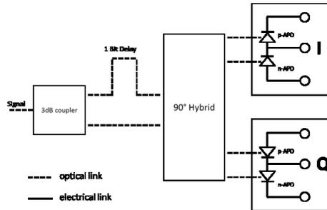
**Fig. 3 Conceptual circuit model of homodyne receiver using balanced APD chips**
