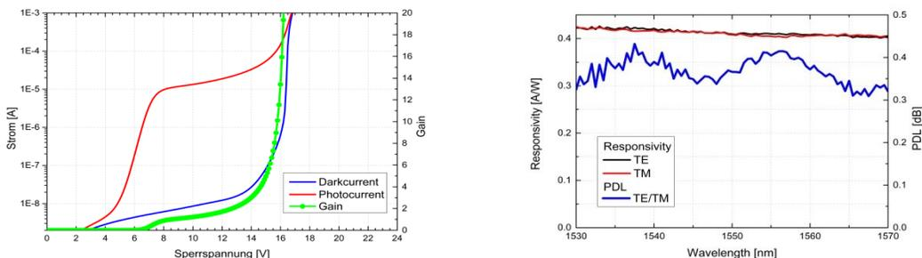
Fig. 1 UI-characteristics (left) and responsivity (right) of fabricated APD chip
