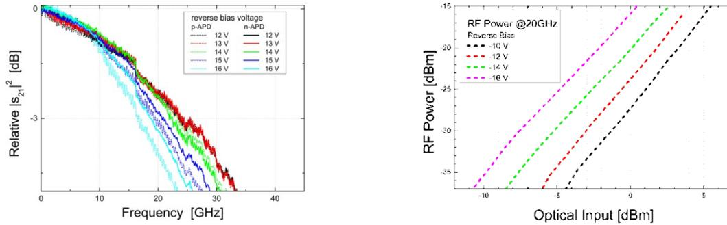
**Fig.2 bias dependent bandwidth (left) and linearity measurement (right) of balanced APD chip**
