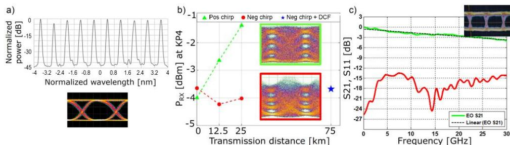
**Fig. 1. a) Output spectrum and typical eye diagram of a 10x10 Gb/s NRZ DWDM TOSA based on the SoC technology. b) Chirp impact on PAM-4 WDM transmission at 25 Gb/s/ $\lambda$  using 10x10G-class TOSA. c) MZM frequency response.**
