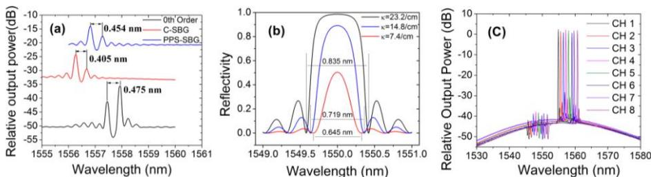
**Fig. 3. (a) Spectra of lasers just below threshold (50 mA) with uniform 0<sup>th</sup> order grating, C-SBG, and PPS-SBG, (b) calculated stop bands of passive laser waveguides, and (c) optical spectra of the laser array.**
