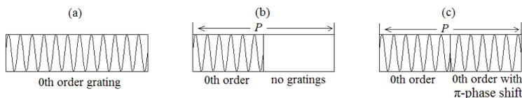
**Fig. 2. Grating structures of (a) uniform 0<sup>th</sup> order grating (b) conventional sampled Bragg grating (C-SBG) (c)  $\pi$ -phase-shifted SBG (PPS-SBG).  $P$  is the sampling period.**
