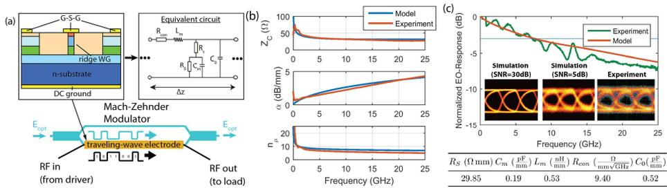
**Fig. 1. (a) Cross section and equivalent circuit, (b) microwave parameters, (c) frequency response, eye diagram and extracted parameters of Mach-Zehnder modulator.**
