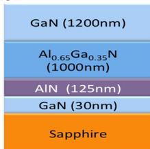
**Fig. 1.** Structure of the MBE waveguide
