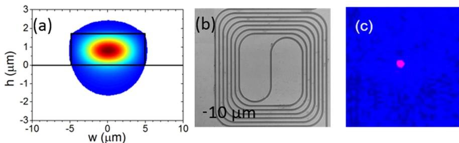
**Fig. 27. (a) Fundamental TM mode intensity profile of waveguide in chalcogenide glasses (width:  $w=10\ \mu\text{m}$  and height  $h=1.7\ \mu\text{m}$ ) at  $\lambda=7.8\ \mu\text{m}$ . (b) Microscope image of a spiral waveguide made of chalcogenide glasses from Ge-Sb-Se ternary system. (c) Propagation-mode near-field in a spiral waveguide at  $\lambda=7.8\ \mu\text{m}$ .**
