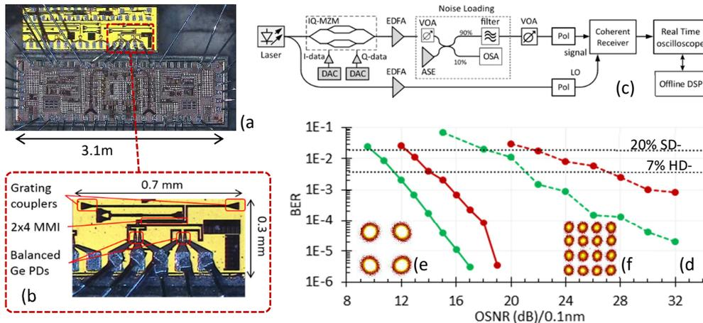
**Fig. 1. (a) Micrograph of PIC + TIA-array chip; (b) PIC layout; (c) Test setup; (d) BER vs OSNR for 28 (green) and 40 Gbaud (red); Example of a QPSK (e) and 16-QAM (f) constellation at 40 Gbaud.**
