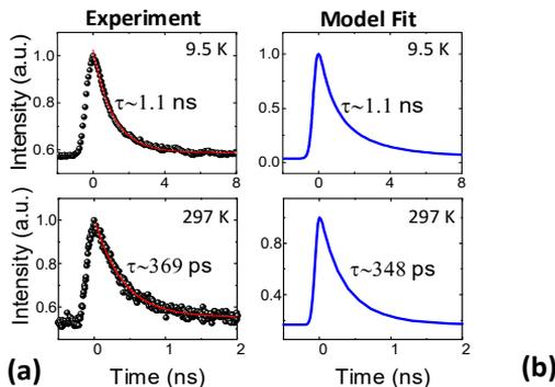
**Fig. 2. (a) Experimental (left) and numerical simulated (right) direct modulation operation at 9.5 K and RT. (b) High-speed modulation at RT varying the bias current revealing sub-100 ps switch-off. In all plots, the modulation was a 80 MHz pulsed signal (100 ps width).**
