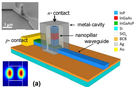
**Fig. 14. (a) Schematic of the waveguide-coupled metal-cavity nanoLED. The inset shows a scanning electron microscope (SEM) picture with the fabricated nanopillar (top-left), and the simulated  $|E|^2$  of the in-plane polarized mode supported by the cavity within the InGaAs active region (bottom-left). (b) Typical L-I characteristics measured at 9.5 K and at RT and model fit (dashed curves). The inset shows a typical spectrum emission at RT.**
