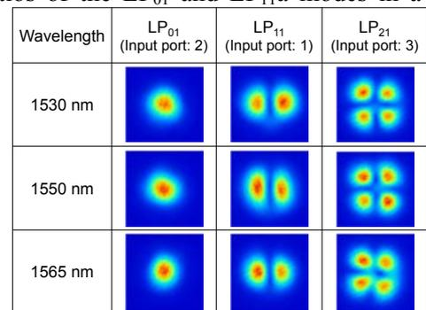
Fig. 4: NFP of output port from each input port.
