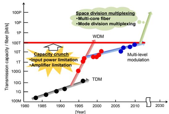
Fig. 1: Increase in single-mode fiber capacity.
