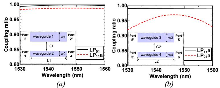
Fig. 3: (a)  $LP_{11a}$  mode coupling ratio dependence on wavelength. (b)  $LP_{21a}$  mode coupling ratio dependence on wavelength.
