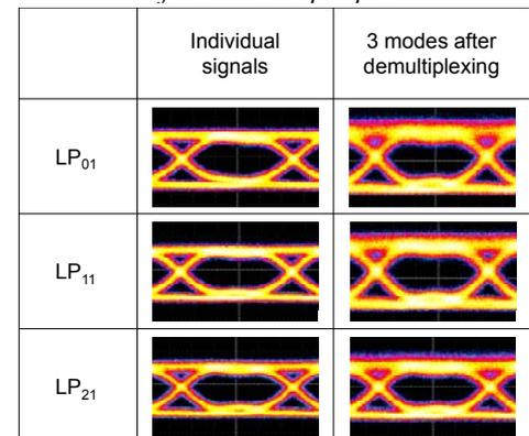
Fig. 5: Eye patterns when inputting signals of individual modes and three multiplexed modes.
