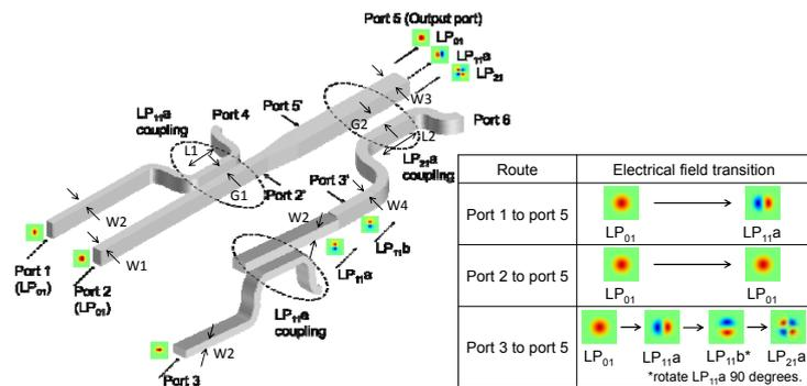
Fig. 2: Diagram of fabricated three-mode MUX/DEMUX.
