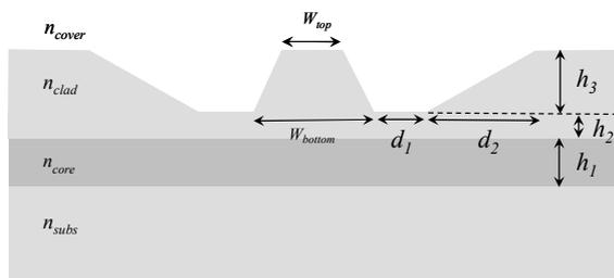
Fig. 1: Transversal section of the ridge structure.
