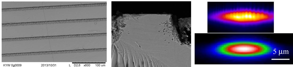
Fig. 3: Left and center: Typical SEM images appearance of the ridge structures produced before end facets polishing. Right: measured (top) and simulated (bottom) waveguide mode at  $1640 \text{ nm}$ .
