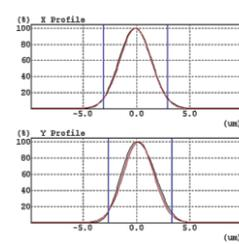
Fig. 4. x-y-intensity profiles of NFP, and Gauss fits @ 808nm
