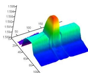
Fig. 2. RI- profile across WG core,  $w=h=6\mu\text{m}$ ,  $\Delta n \sim 0.0050$ , @ 678nm
