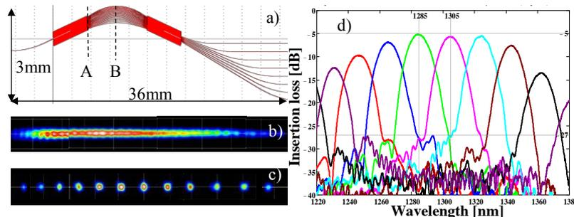
Fig. 5. a) 1x8 CWDM design; b-c) Int. distribution in front (cut A in 5.a) and middle (cut B in 5.a) of the AWG; d) Spectral transmission at the output ports 1-8 using Super-Continuum-Laser @ 1200 – 1400 nm
