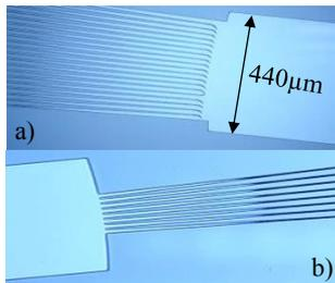
Fig. 1. Pictures of CWDM parts; a) AWG out at star coupler, b) 8x WG output
