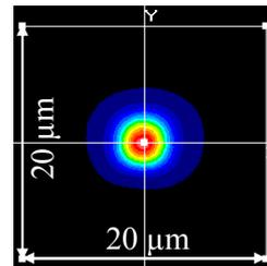
Fig. 3. NFP of a SM-WG,  $\omega_{x,y}=5.9\mu\text{m}$  ( $1e^2$ ), @ 808nm
