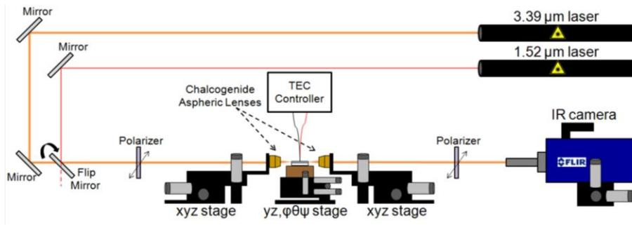
Fig. 2. Scheme of the optical setup used for modal characterization of NIR and MIR waveguides
