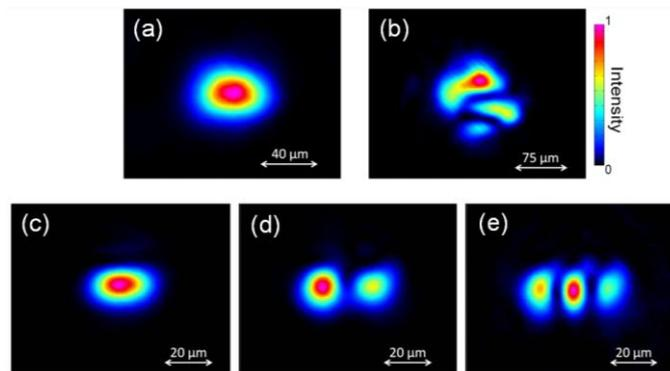
Fig. 3. Measured near-field intensity mode profiles for selected waveguides at 3.39  $\mu\text{m}$ . (a) Monomode and (b) multimode waveguides made in  $\alpha$ -quartz. (c), (d), (e) First three modes supported by a step-index waveguide made in fused silica.
