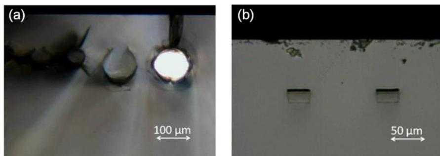
Fig. 1. Microscope images of fabricated waveguides in (a)  $\alpha$ -quartz crystal and (b) fused silica glass.
