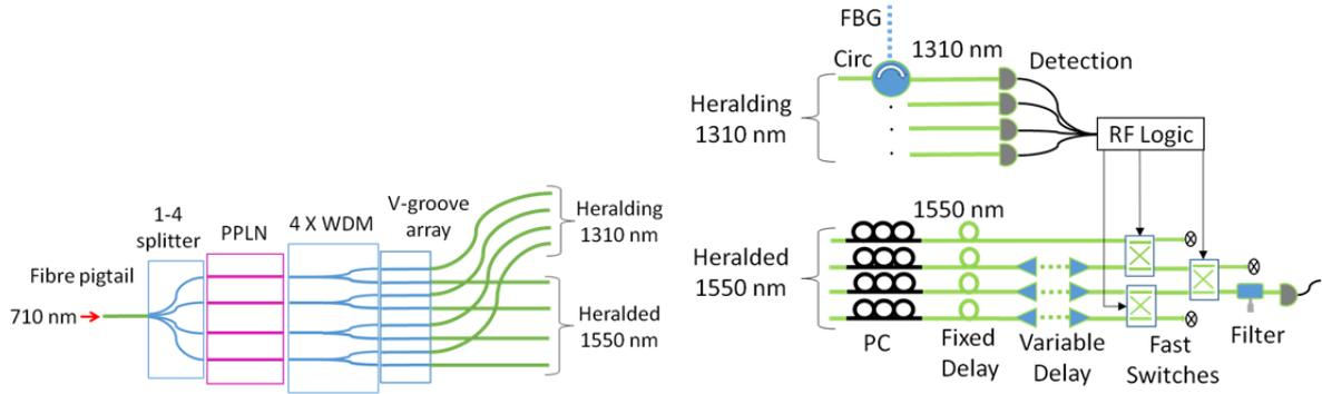
Fig.1: (left) A picosecond laser pumped array of 4 identical PPLN waveguides, where a pair of FLDW chips couple light in and out of the device. (right) The output of the WDMs is sent to a multiplexing setup. Four single photon channels at 1310 nm, which are filtered by FBG and circulators (Circ), herald the arrival of 1550 nm photons. Radio frequency (RF) electronics control the switches for routing the 1550 nm photons.
