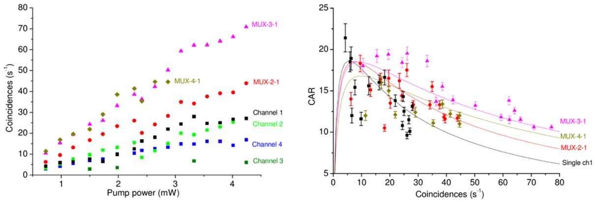
Fig.2: (left) Heralded photon rate vs. pump power for single channels and a 4-1 multiplexing scheme. (right) CAR vs. coincidences for multiplexing 2, 3 and 4 channels. Single channel 1 is shown for comparison.
