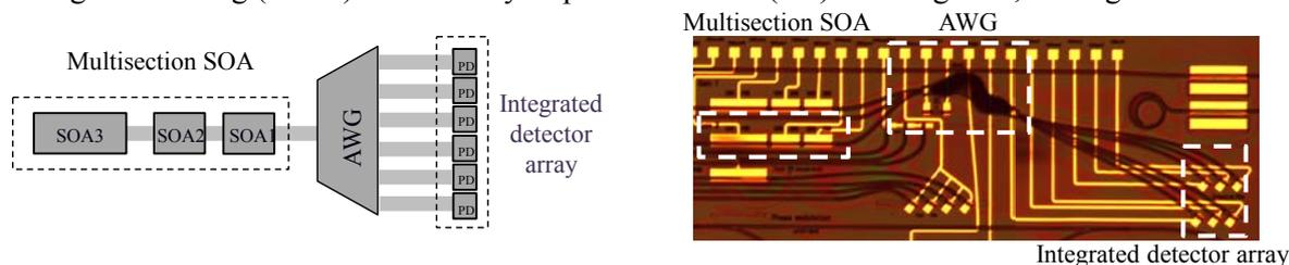
Fig. 1 Schematic of the integrated modal gain measurement (left) and a microscope photograph of the realized circuit (right).
