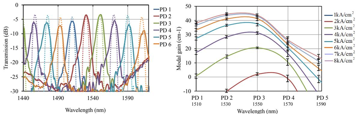
Figure 2 Measurement (cont.) vs. simulation (dashed) AWG transmission (left), and modal gain with error bars (right).
