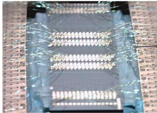
*Fig. 1: Photograph of the 16 × 16 optical switching matrix. Chip dimensions are 4 × 14mm<sup>2</sup>.*
