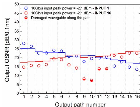
Fig. 3: Path dependent noise performance. Experiment (symbols) and prediction (solid lines).
