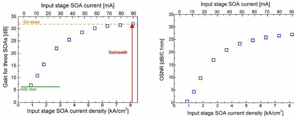
Fig. 2: Gain for three SOAs (a) and optical signal to noise ratio (b) for path 1 to 1 as a function of injected current at the input SOA. The central and output SOA currents are set at 90 mA and 160 mA, respectively.
