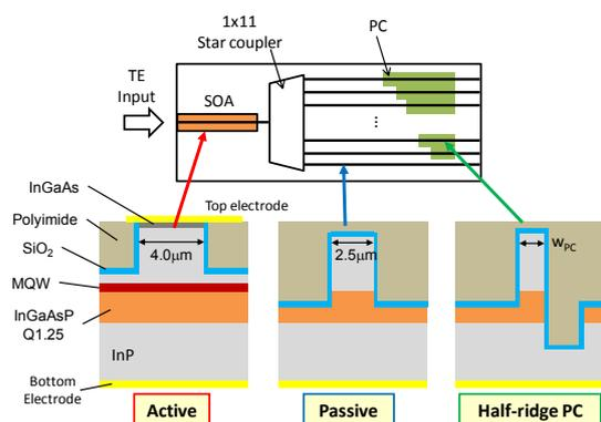
Fig. 3: Schematic of the fabricated PIC with half-ridge PCs and MQW SOA integrated on a single chip.
