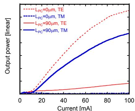
Fig. 4: Measured output power of the TE (red) and TM (blue) components of the light from the ports with PC (solid lines) and without PC (broken lines).
