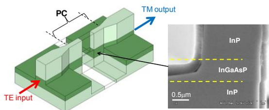
Fig. 1: Schematic of half-ridge InP/InGaAsP PC and SEM image of the fabricated device [8].
