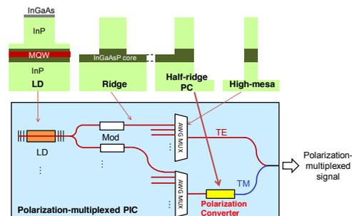
Fig. 2: Schematic of polarization-multiplexed PIC.
