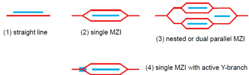
Fig.2 Evolution of Ti:LiNbO<sub>3</sub> MZI modulators
